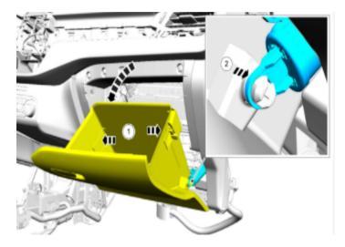
2. Remove the screws and open the cabin air filter door.
