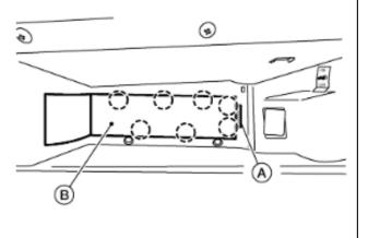
• Release in-cabin microfilter cover tab (A) in direction shown, then remove in cabin-microfilter cover (B)
