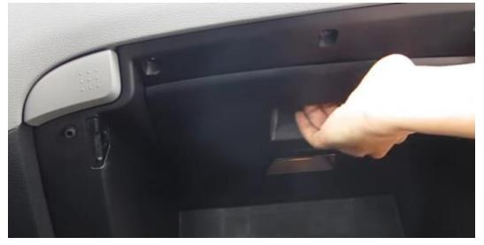
3. Remove the cabin air filter cover by pressing upwards on the bottom clips
