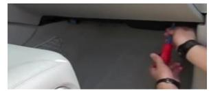
2. Open the glove box, remove the cover panel from the right side, and remove the screw at the bottom right
