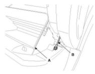
3. Remove the filter cover (A) push the tabs in and pull. Remove the old cabin air filter, taking note the air flow arrow indicator direction on the side of the old filter.
