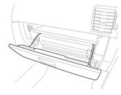
2. Remove the glove box(A) from the lift(B).
