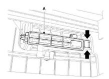
4. Insert the new filter (B) into the housing, making sure the air flow direction is correct according to the arrow indicator.
