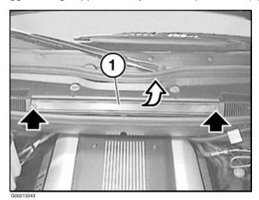
3. Pull out the old filter (1) in direction of arrow. Clean the housing
