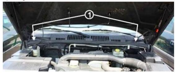
2. Open the hood, remove 2 screws securing the housing cover and remove the cover. Pull out the old filter, clean the housing and insert the new filter
