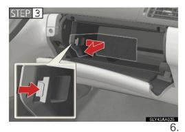
Locating Glove Box Partition Remove glove box cover. See step 3
