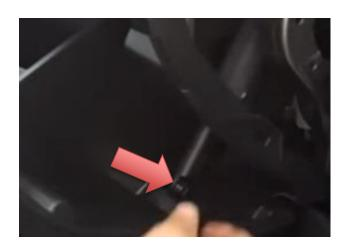
2. Remove the cabin air filter cover by pulling down on the two tabs and pulling out.
