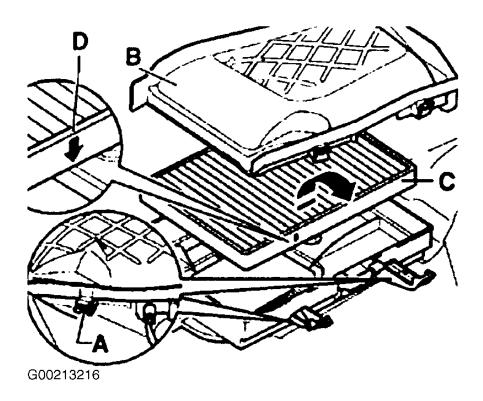
9. Make sure the rubber seal is fitted properly and it is securing the cowl plastic cover.
