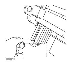
Remove the first filter by pulling the filter tab. See ←
