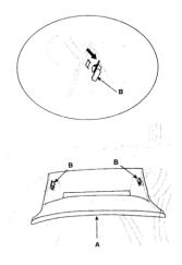
2. Remove the side <u>damper</u> (A) from the glove box.
