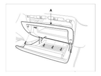
2. Remove the filter cover (A) with pushing the knob.
