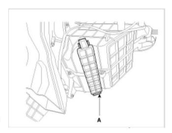
3. Replace the air filter (B), install it after making sure of the direction of air filter.
