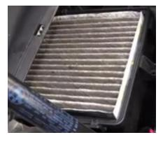
Reverse steps 4-1 to reinstall with arrows facing towards each other (bottom filter up and top filter down).
