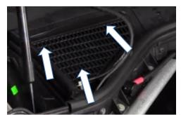
Remove the cover by squeezing the tabs together and lifting.
