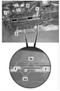
3. Remove both combination filters (4) downward out of air conditioner housing (3)
